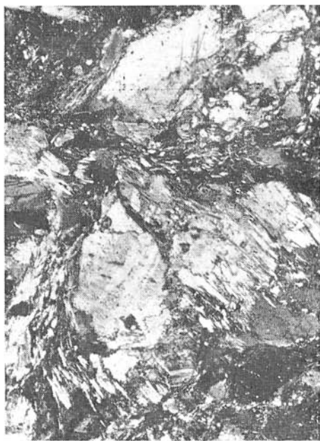
Fig. 4. Porphyroblastic structure of albite-actinolite schist [albite — light green amphibole] — the Nižný Klatov — Zlatá Idka roadcut. Magn. 48 x, X pol.
